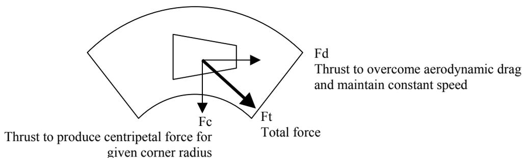
When the car is cornering at the maximum speed, the total force  $F_t$  will be equal to the maximum force that can be transmitted through the tyres:
