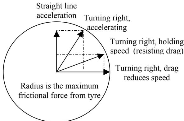
As the speed increases, the centripetal force (lateral acceleration) increases, and there will come a point where the result of the two perpendicular forces equals the maximum frictional force. We are now at the limit of the tyre's grip.
