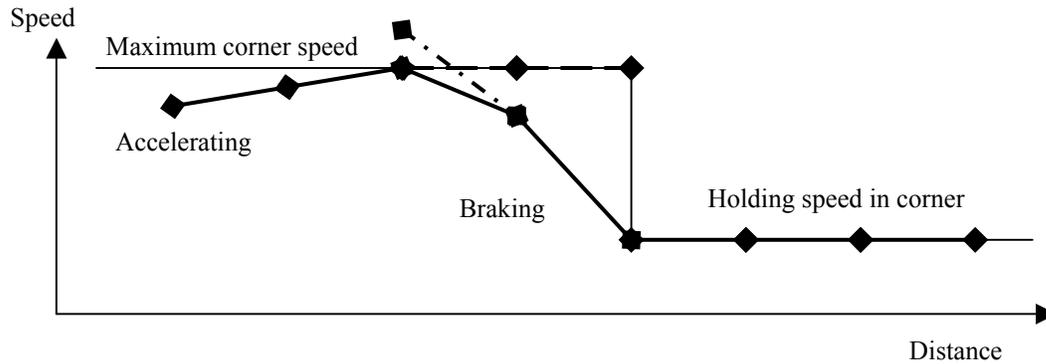
The initial calculation of maximum corner speed and forward acceleration can be done by progressing forwards through each sector in turn, feeding the exit velocity from one sector into the entry velocity of the next. To calculate the best possible braking performance, we will first calculate the acceleration from rest and maximum corner speeds, then apply the braking forces on a second pass, this time going backwards through the sectors.
