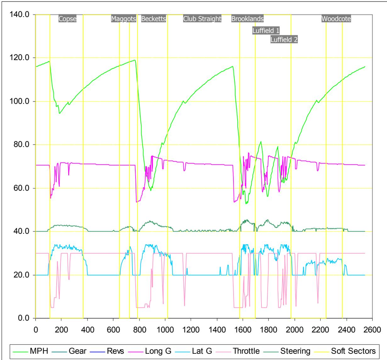
It should be noted that the lateral G and steering graphs only go in one direction, since the model cannot currently distinguish between left-hand and right-hand corners! This would only be a problem if we wanted to directly compare the results with real car data.
