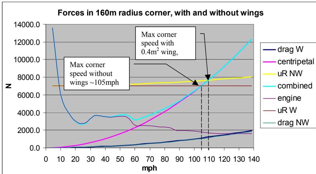
The wing will add extra drag to the car, again this is calculated using the coefficient of drag and the plan area of the wing:
