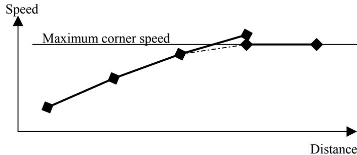
In reality, the driver would continue to accelerate until the maximum corner speed was reached, then hold that speed. As our track is split up into sectors, we can model this as shown in the diagram, where the exit speed is simply set to the maximum corner speed. The average acceleration will be the same regardless of how we model the transition, since the entry and exit speeds will be fixed.
