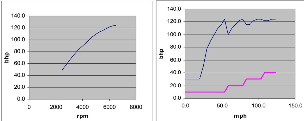
Again, this method could also be used given the torque curve of the engine. It is difficult to model the effect of gear change time using this method. When the engine is not accelerating the car, the car will slow down the revs will drop, and oscillation can occur on upshifts unless some hysteresis is introduced.
