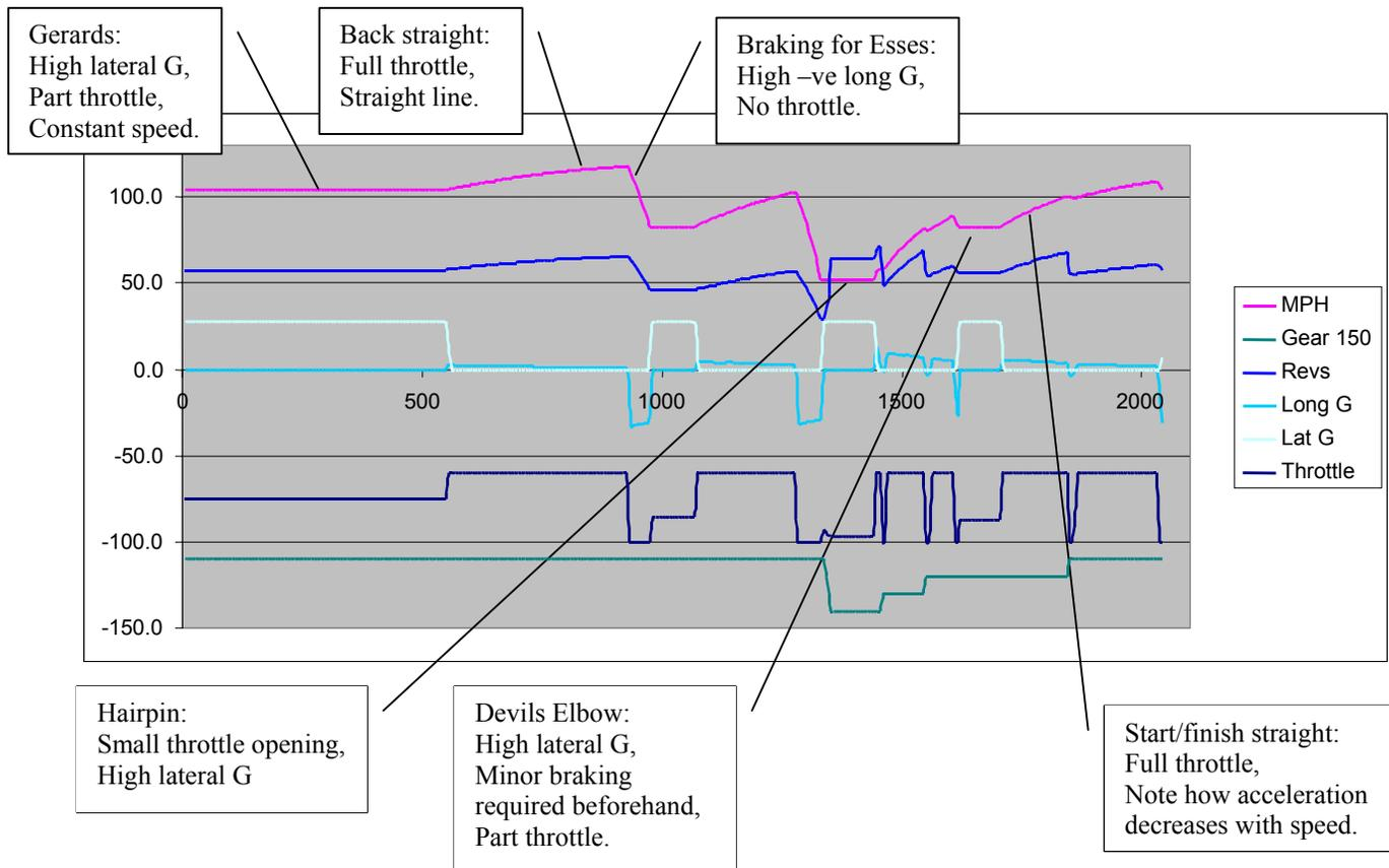
We can see that the driver is making the best use of the tyres in this example under both cornering and braking. As this simple track has constant radius corners, the lateral G loading and throttle opening are
