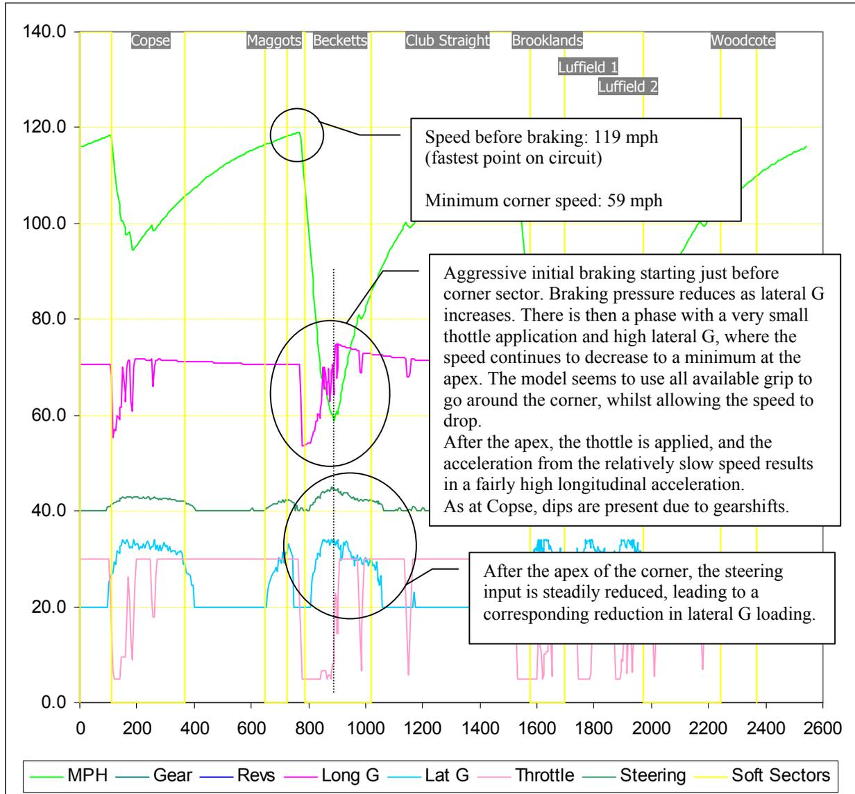
In the real data trace, the driver does most of the braking prior to the corner, and turns in with a balanced throttle. The steering lock and throttle remain fairly constant throughout the short corner, after which full throttle is applied and steering lock reduced. Incidentally, the real data shows serious power-on oversteer on the exit of this slow corner!
