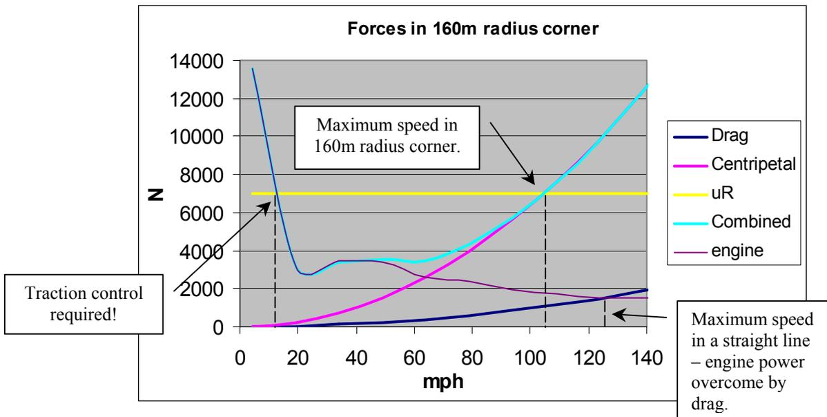
At slow speed, the available force from the engine would exceed the maximum frictional force and cause wheelspin if all the power was applied. At higher speed, it can be seen that the centripetal force becomes the dominating factor. The maximum speed is reached when the combined force is equal to the maximum frictional force. We can also see from the diagram that the maximum straight-line speed would be reached when the drag force becomes equal to the accelerative force from the engine.
