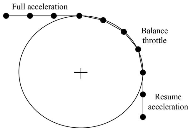
While accelerating in a straight line, the force produced by the engine (longitudinal acceleration) will often be less than the maximum frictional force. Exceptions to this might be a grid start, or a Formula One car running on cold tyres. It should therefore be possible to negotiate a corner whilst still accelerating.
