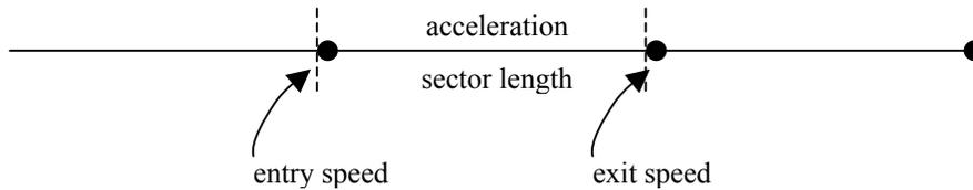
If the car is accelerating from rest, we can take account of the available grip from the tyres, the engine power and aerodynamic drag and calculate the acceleration possible at the start of each new sector. From this, we can then calculate the exit speed at the end of the sector, given the length of the sector and the assumption that the acceleration is constant.
