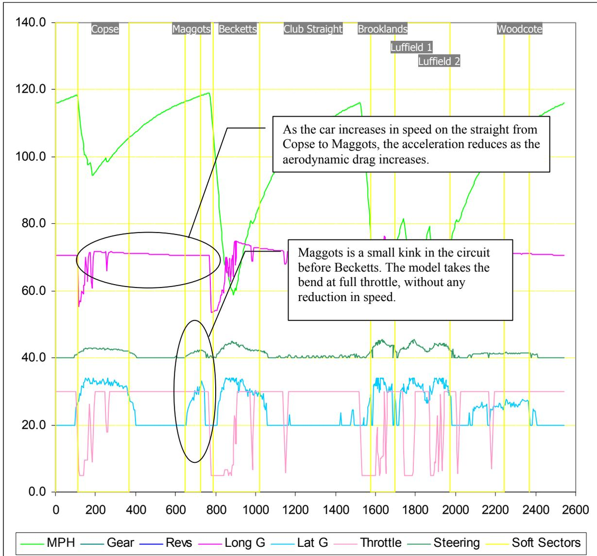
In reality, Maggots presents a challenge for the driver since it is on the brow of a slight hill, and there is a large amount of braking to be done before Becketts – which is hidden over the hill. It is very tempting to lift of the throttle on the entry to Maggots.
