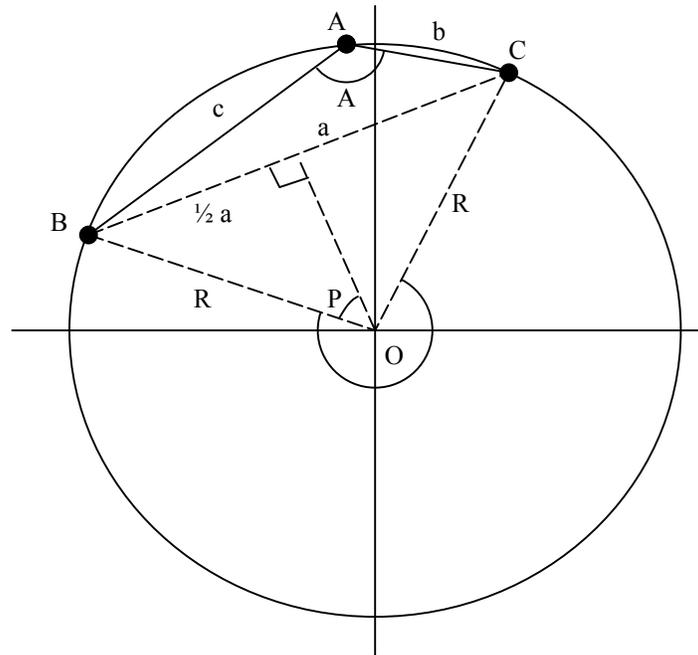
Having drawn three points A, B, C on a circle whose centre is at O, we know from a circle theorem that the exterior angle BOC is twice the interior angle A (BAC).
