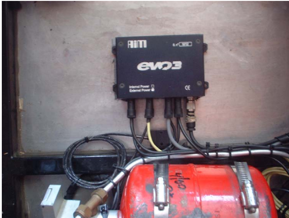
The box is attached with Velcro – soft side on the car, hooks on the box.
