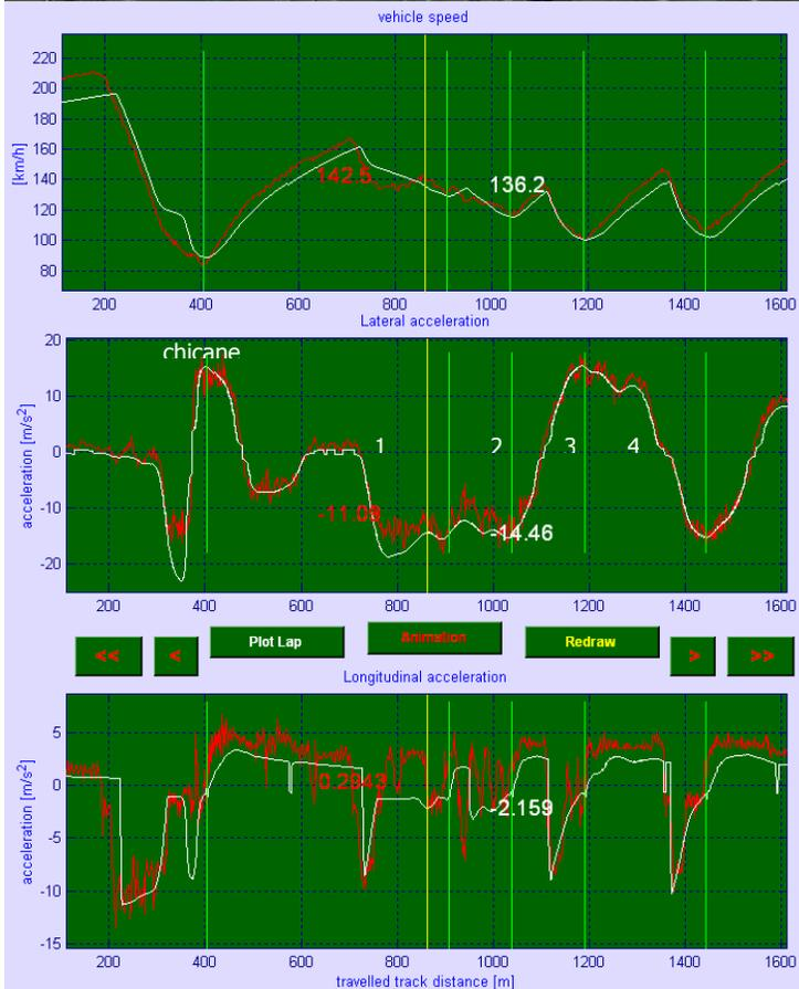
From the accelerations trace below it can be seen that the braking area for turn 3 is at a point where the car is changing from a right to a left turn – trail-braking and good transitional (i.e. shock) performance is required for a good balance here.
