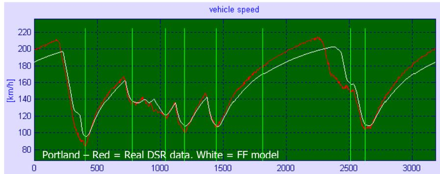
The suspicion is that something has gone awry with the combination of measured lateral G and wheel speed used to generate the track model. The wheel speed has been scaled (+2.55%) to ensure the proper track length – this would affect the calculated corner radius. However, the map produced from the unscaled speed data generates very similar results. We will therefore look for a problem with the lateral G input.
