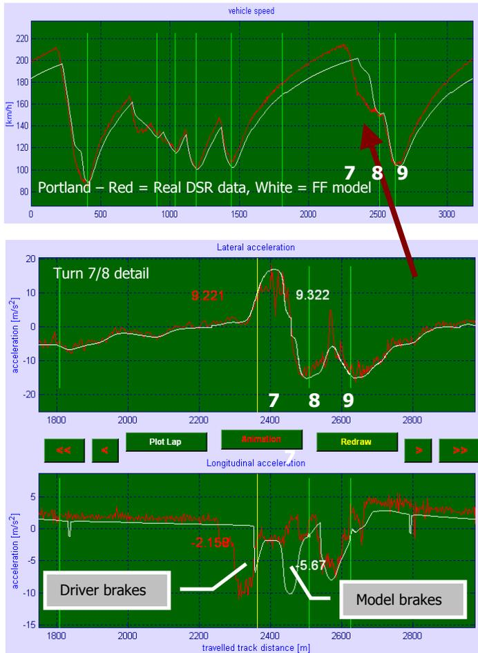
Looking at the comparison of the FF model with the real DSR data, it can be seen that the model is more aggressive on corner entry where there is a complex combination of braking and cornering required – especially going into the chicane and turn 7/8.
