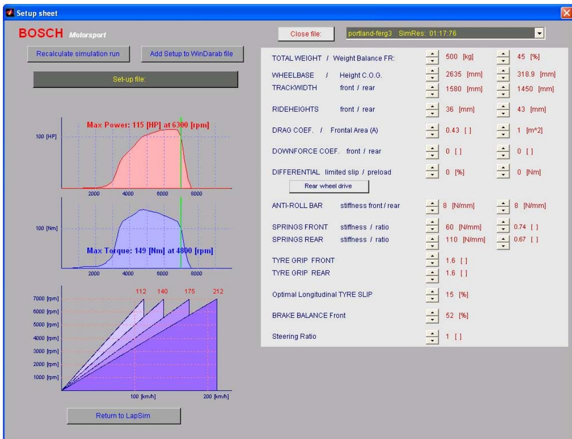
In the model data above, the roll bar figures are known to be inaccurate, but that should not greatly affect the overall lap time.
