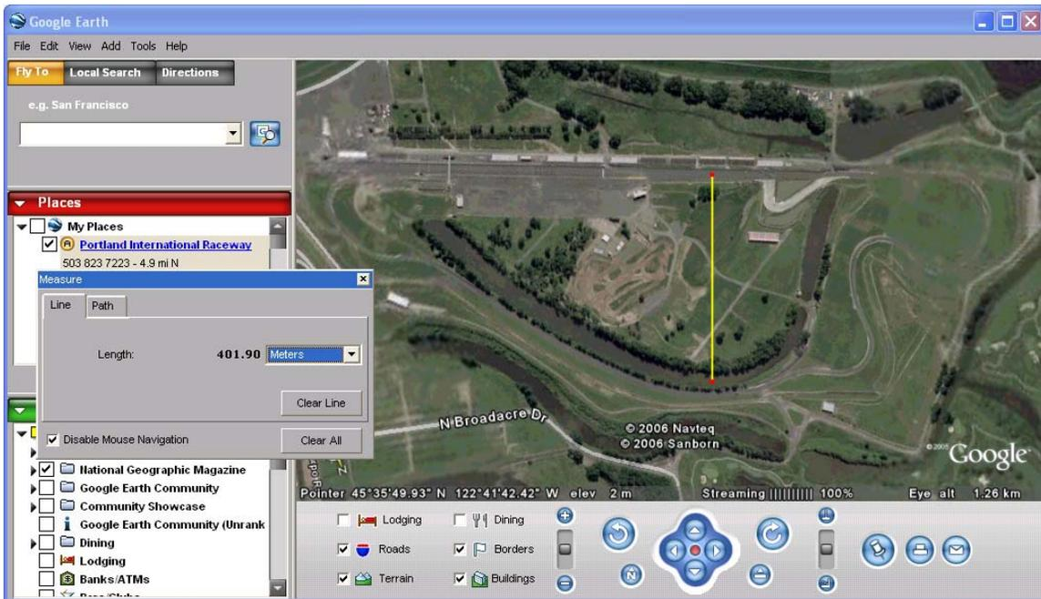
The same measurement made using Google Earth also appears to be around 400m – so the correction factors applied to the map now seem reasonable!
