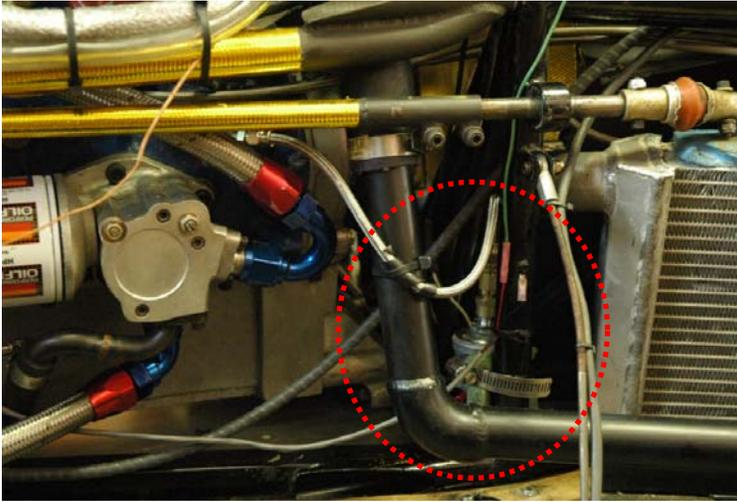
A VDO 0-10 bar pressure sender is used for oil pressure, mounted remotely.
