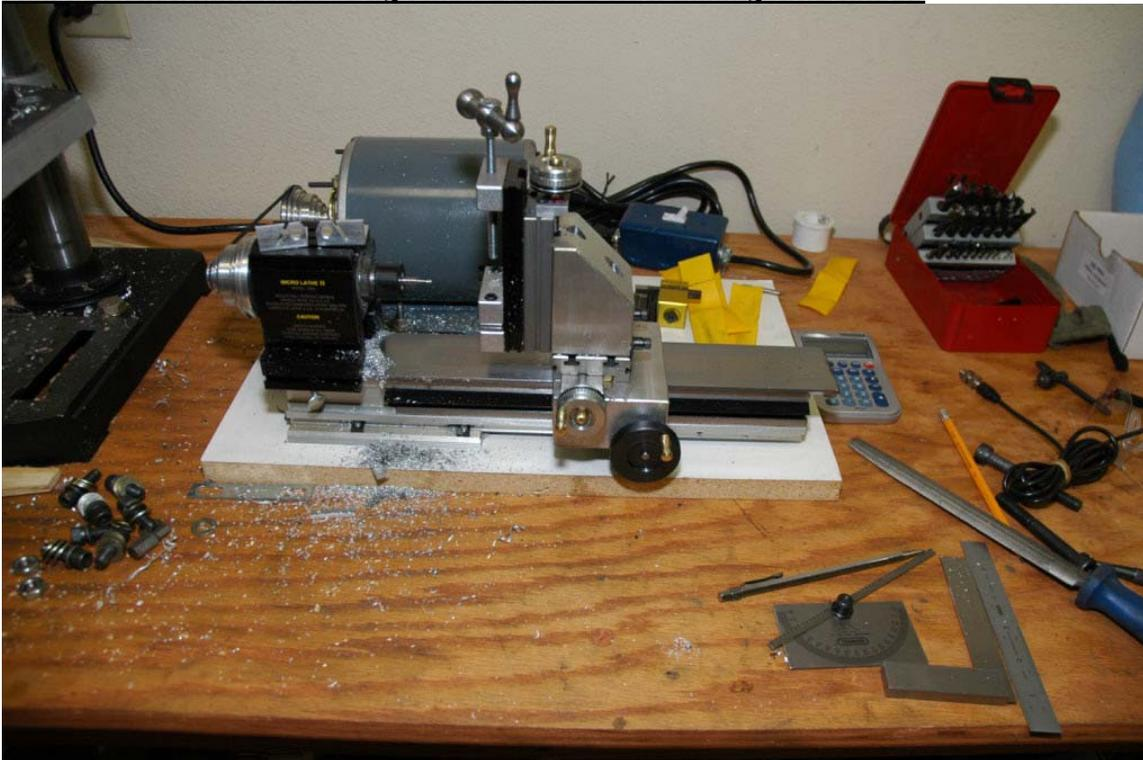
The tiny benchtop lathe/milling machine used to create the various brackets and spacers required. It's small, but big enough for many urgent or would-be-nice jobs – and relatively inexpensive at \$650 for the machine, motor and a variety other stuff like the milling attachment, chucks, end-stock, cutters, milling vice, cross-slide etc.
