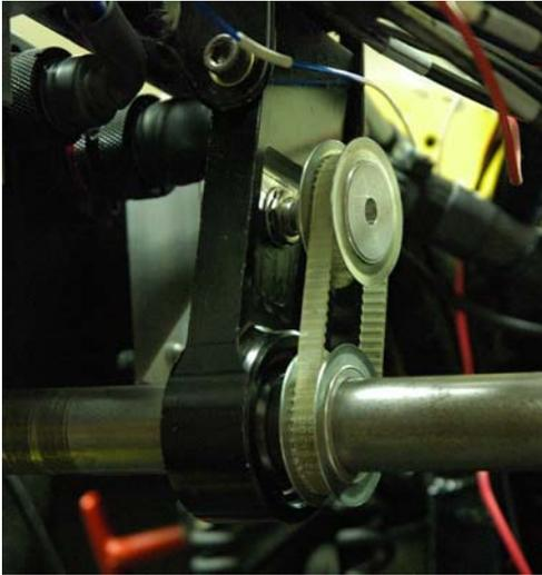
Another Bourns 6639S-1-103 pot is used – this time mounted directly to the steering column support block. The pot is operated by a 1/4" wide toothed belt connecting pulleys on the steering column and the pot.
