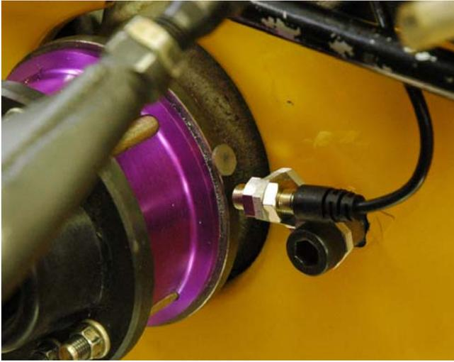
Speed is measured on both sides at the rear at the inboard tripod joints.
