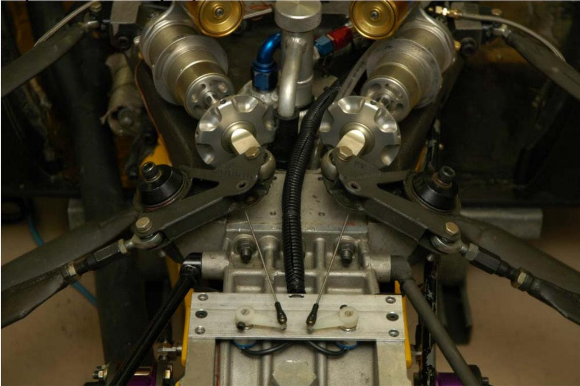
The rear suspension movement sensors are once again Bourns pots (6639S-1-103). The hardware is the same as that used on the throttle – radio-control aircraft control linkages. This setup requires a bit more care than the front sensors, as it is possible to damage the linkages if the spring is removed and the wheel is allowed to drop. The linkages are mounted on the underside of the bellcrank, at a position to give a reasonable range of motion at the lever.
