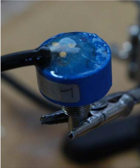
Each of the Bourns potentiometers used is protected with 5-minute epoxy – after the wires have been attached and the sensor tested, epoxy is used to seal the connections and provide strain relief for the cable.
