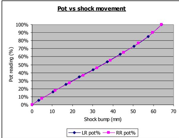
As can be seen in the chart to the left, the relationship between shock movement and pot movement is fairly linear, but goes non-linear towards the end of the shock travel – due to the design of the linkage.
