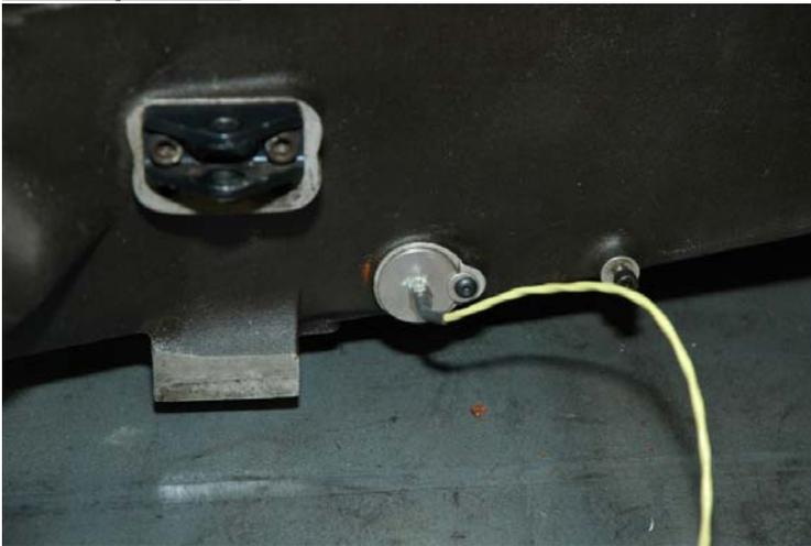
An M5 thermocouple (from AIM) was used – mounted in the left side of the oil tank. A hole was drilled and tapped into a plug used to fill in a hole in the side of the tank. The corresponding hole on the opposite side is used for the oil pump pickup line.
