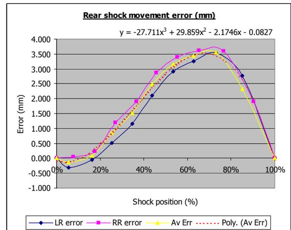
If the position of the pot levers to the suspension were changed (e.g. change of length of the linkages), this calibration would have to be repeated.
