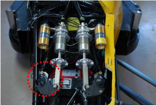
A Bourns 6639S-1-103 pot is used, mounted to a piece of 1 1/2" x 1/8" L-section aluminum, glued to the frame with 3M 2216 epoxy. The mounting surface of the L-section was machined to add an 8 degree slope to nicely match the shape of the box section in the frame.
