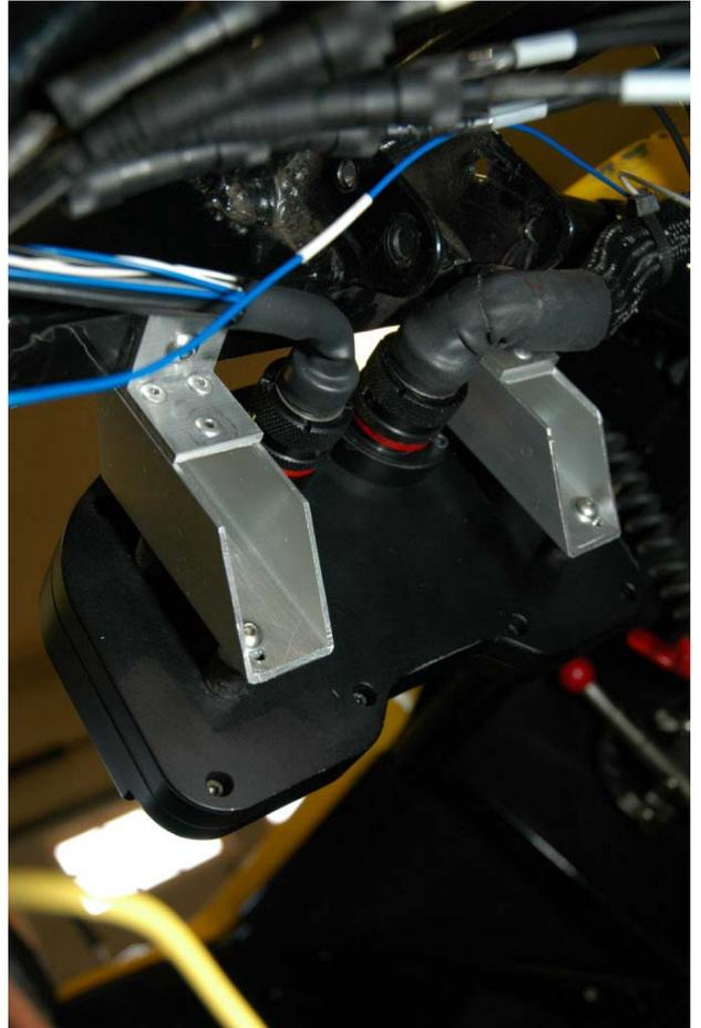
It was necessary to create a second wiring harness for the 22-pin Deutsch connector – in order to accept inputs for wheel speeds 3 and 4. The harness also allows for remote control of the MEM and VIEW buttons, plus an external USB connection, and ECU interfacing via CAN and RS232. In due course, a button for VIEW may be placed on the steering wheel.
