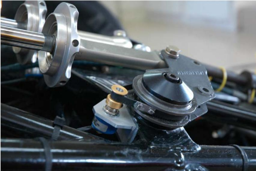
The pulley on the pot is also MXL from McMaster, and allows the range of suspension movement to drive the pot through approx 270 degrees – for great analog-to-digital sensitivity.
