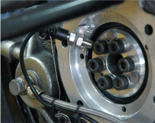
Speed is measured on both front wheels.
