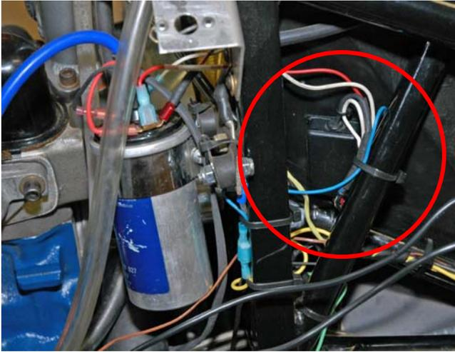
The RPM signal comes from a filter box attached to the LT side of the coil. The box came with the car – and it looks fairly home-made inside. The output signal from the box is connected to the low-voltage input on the dash.
