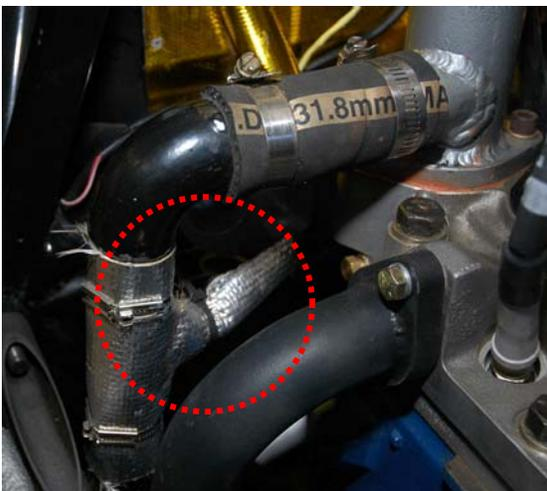
The water temperature sensor is another M5 thermocouple, mounted in a pipe between the left-side radiator and the thermostat housing.
